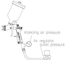
Pulling the trigger of the gun with the pattern adj. set and air adj. set fully opened, adjust the air regulator in the spray booth to obtain 1.0~1.1 bar (14~16 PSI) at the gun inlet as issued on specifications table ahead. In this way the gun will atomize within 0.7 bar (10 PSI) inside air cap.
