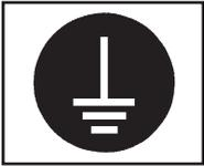
Securely ground the unit, spray gun, workpieces and containers containing paint or solvent. Be sure to use ground wire set supplied with Airless Unit. Connect it to ground to have continuous grounding.
